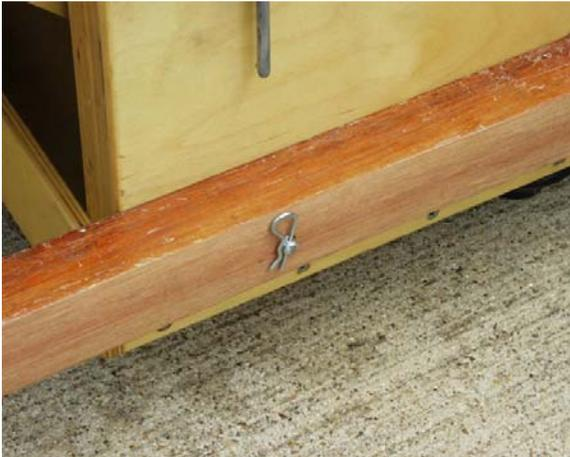
To complete the project, I screwed the pins into the threaded inserts in the rocker box then slid on the handles. 7/64" x 1 5/8" hitch pin clips through the holes keep the handles from coming off while moving the scopes. With the new pins, we have virtually eliminated the time it takes to connect and disconnect the handles. Since its so fast and easy we now use a single pair of handles for both scopes.
