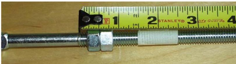
The first task was to shorten the threaded section of the bolt to 1 1/2". I first threaded a couple of nuts onto the bolt past the cut point. If the cut is clean, the
