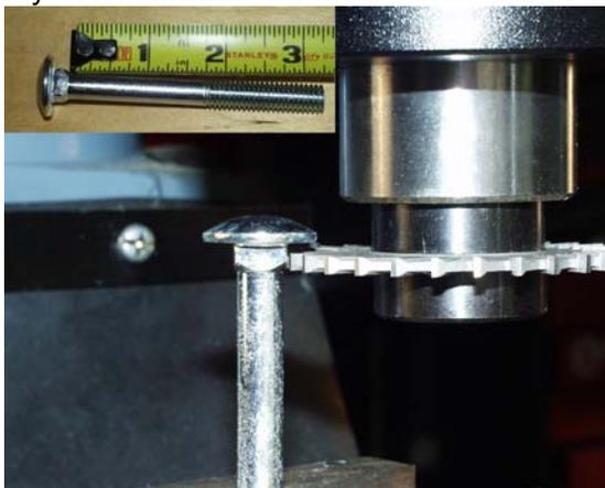
The last task to fabricating the pins was to drill a 7/64" hole approximately 1/8" from the end of the pin. I used two tools to make this job a snap. The first is a drill press. If you don't have one and your significant other won't let you buy one, then borrow one. Only
